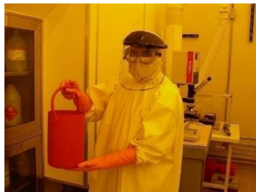
4. Finish with chemical gloves. Note transfer bucket
