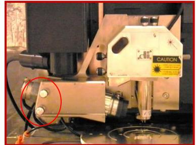
Focus on tip using the trackball.
