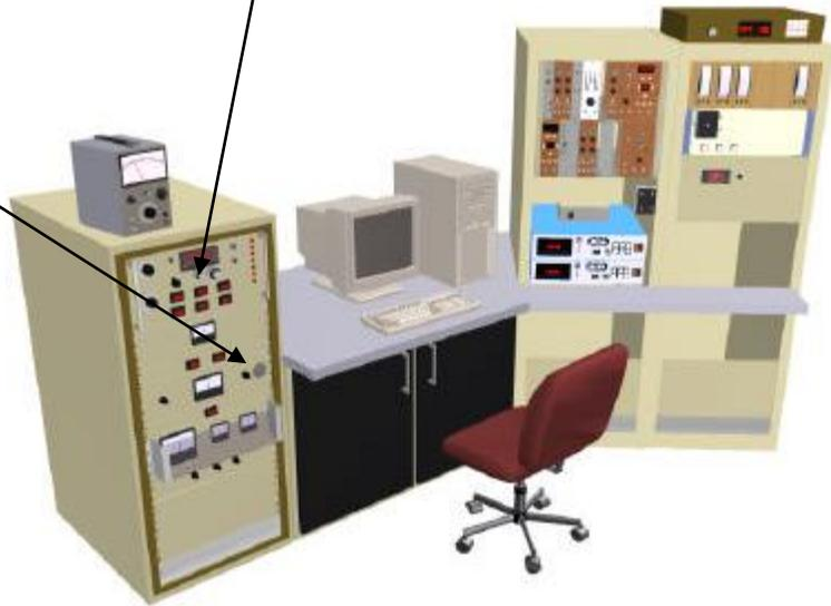
5) Continue to increase or decrease the terminal voltage in 20 kV steps, adjusting the magnet setting each time. Each time you have incremented the terminal voltage by 100 kV, adjust the following parameters, one at a time, to maximize the beam current on the electrometer.
