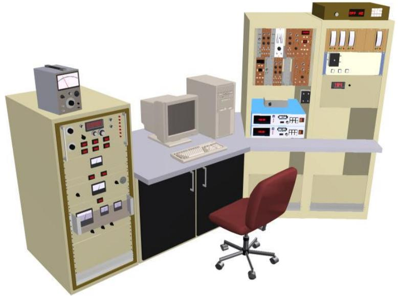
4. Connect the ammeter to the BNC connection for the copper target block inside the PIXE line. (Rotate target block to block beam)
