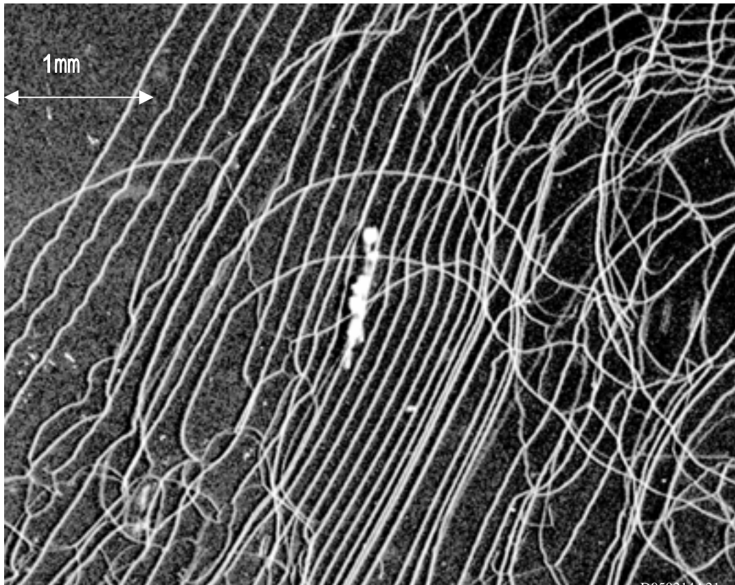
Fig. 6.3 Example of extinction contrast (positive) topography of dislocations in Si crystal
