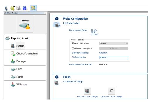
17. If you are using NCHV-A probe, at the next screen, select Auto Tune. Not necessary for ScanAsyst probes.
