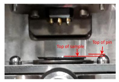
6. Insert probe holder completely into *Head*, taking great CARE to clear the sample. Allow it to fall onto the reference pins. Tighten clamping screw on back of Head to secure probe holder.
