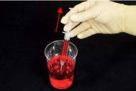
Insert supply syringe into fluid container with the plunger fully depressed. With the syringe still inserted, slowly pull plunger until syringe is filled. Remove syringe.
