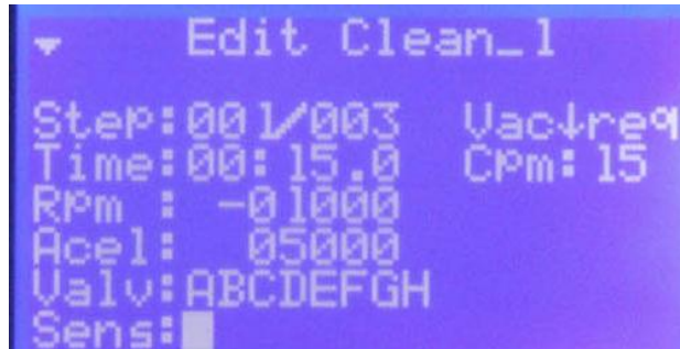
Figure 3-27 EXAMPLE OF NEGATIVE SPIN SPEED VALUE
