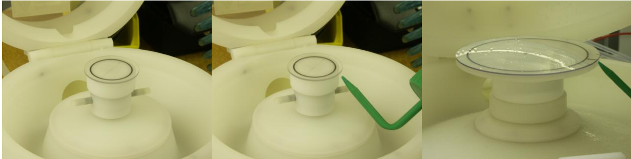
Figure 4-2 Wet Testing 1.75" and 200mm Chuck
