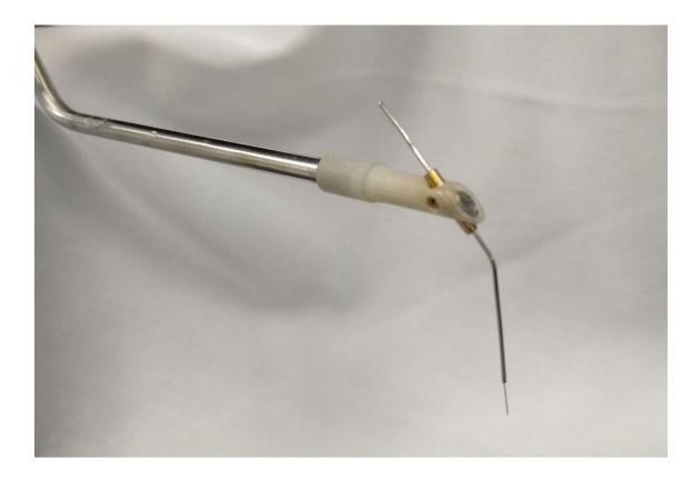
In addition to adjusting the needle in / out, you can bend the needle as shown if you need better access to your device contacts. This may occur if you are trying to fit multiple contact needles onto a small area of your sample.
