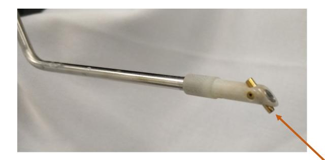
The probe needle goes into this socket. It is a friction fit – simply push in / pull out.
