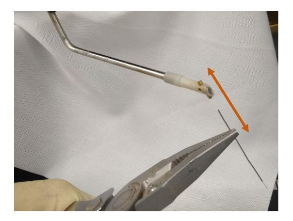
You can use a needle-noise plier or tweezers to insert / remove the probe needle from the socket on the end of the probe. The probe is held in place by friction. Be sure to align the probe with the socket and it should insert with minimal force.
