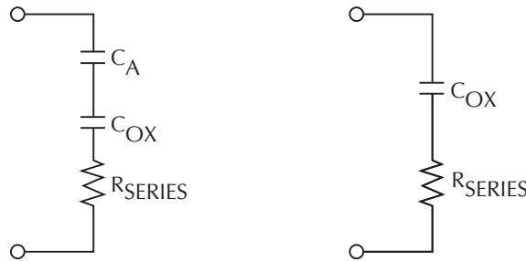
A. Equivalent Three Element Model of MOS Capacitor in Strong Accumulation
