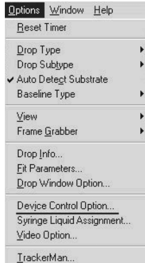
Fig. 3.1: Selection of the menu item "Device Control Options..." from the "Options" menu
