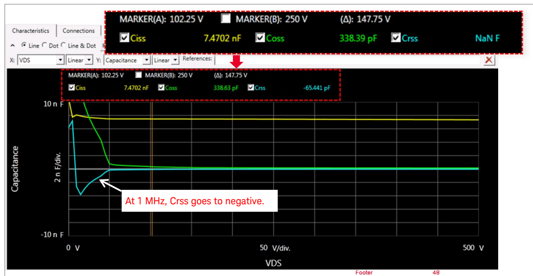
Figure 4-20 Crss measurement example (linear Capacitance scale) at 1 MHz (super junction FET).
