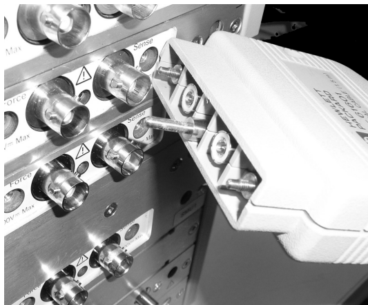
Figure 2.18. The Kelvin triaxial cable mates with Keysight SMUs and many analytical wafer prober connector plates.
