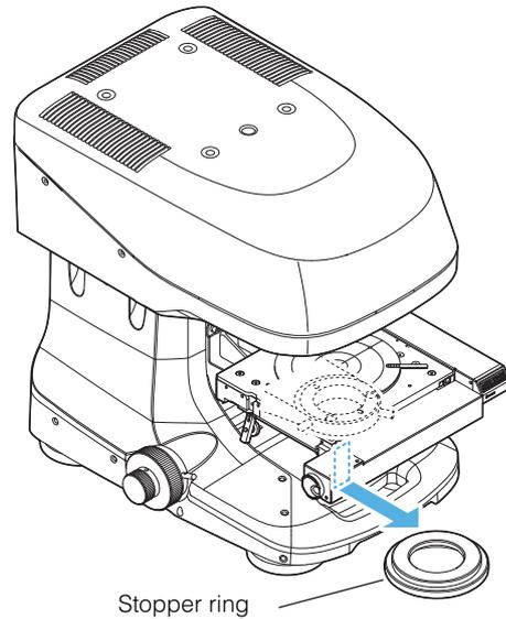
**3** Remove the motorized XY stage from the stage base, and attach the removed stopper ring on the bottom of the motorized XY stage.
