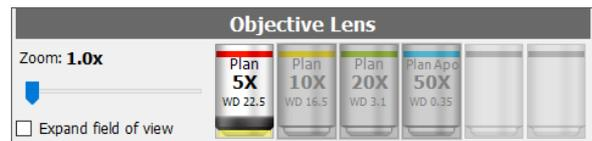
The revolver rotates automatically and the selected objective lens moves.
