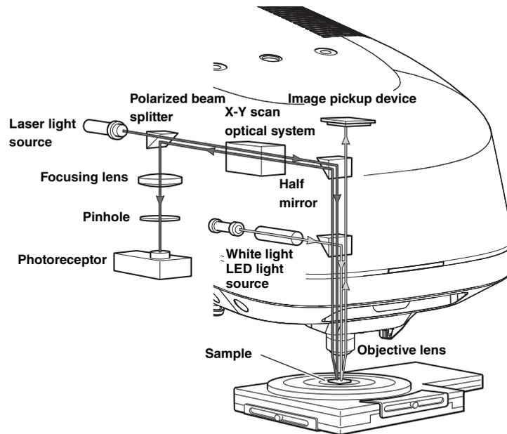
The light emitted from the laser light source is focused onto the surface of the sample via XY scan optics and objective lens. The focused spot light scans the image area within the field of view using the XY scan optical system.
