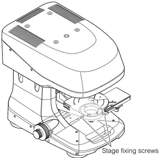
**3 Remove the standard XY stage from the stage base, and attach the removed stopper ring on the bottom of the standard XY stage.**
