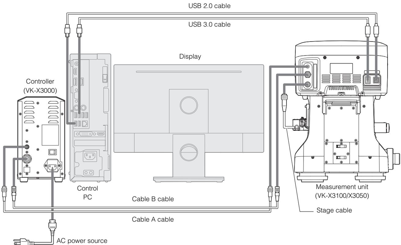
**WARNING** Be sure to connect the power cable to an outlet that has a grounding terminal.
