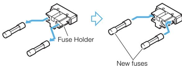
**5 Insert the fuse holder back into the power connector.**
