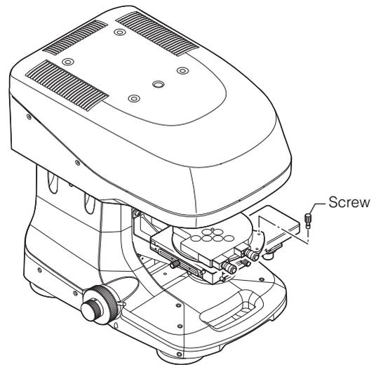
**4** Insert the protrusion on the base of the rotating stage into the recess in the center on the top of the tilt stage.
