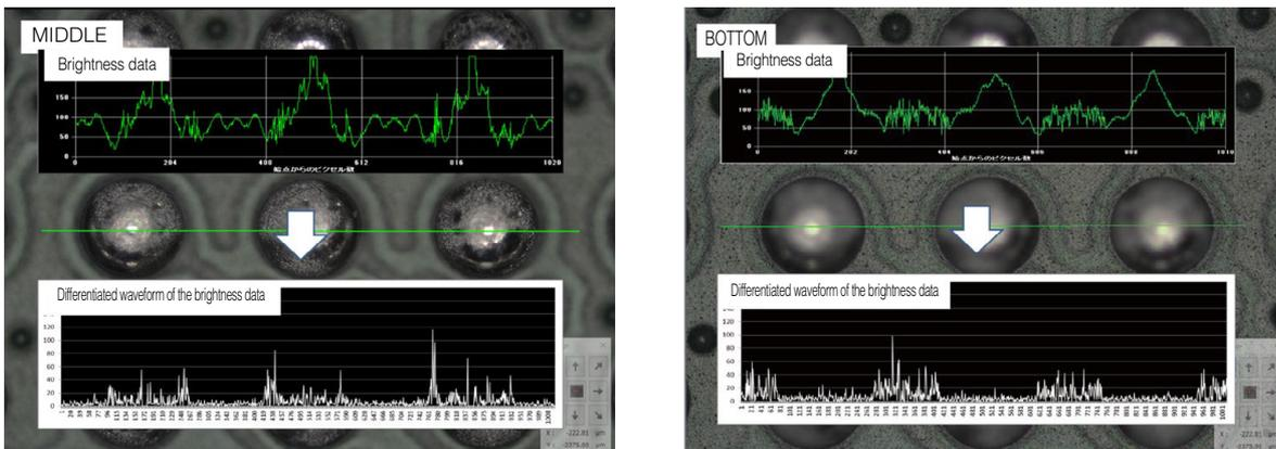
Focus variation focuses on the camera's high-contrast pixels and the pixels around those pixels. The brightness difference between adjacent pixels is recorded while the objective lens moves up and down.
