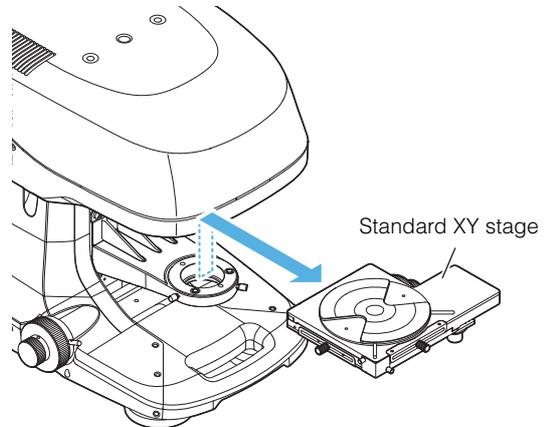
**4 Tighten the stage fixing screws.**
