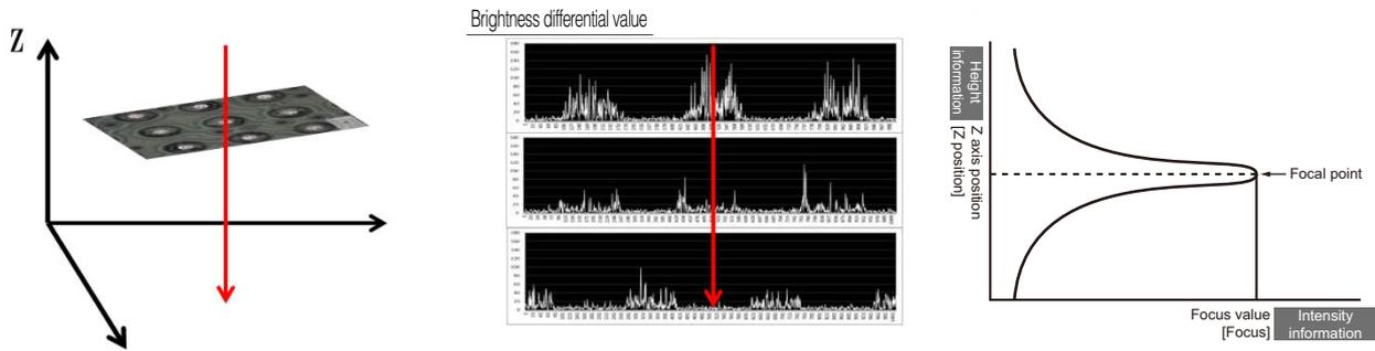
By converting the image luminance difference (amount of image blurring) caused by the objective lens moving to a focus value and making a graphical representation of the vertical movement (positional data of the linear scale) of the objective lens, you can obtain the focus data for each Z position like shown in the above figure.
