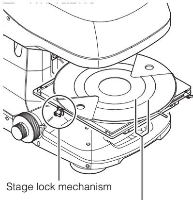
When observing a 6- or 8-inch wafer, align the wafer to the edge of the stage and fix it there.
