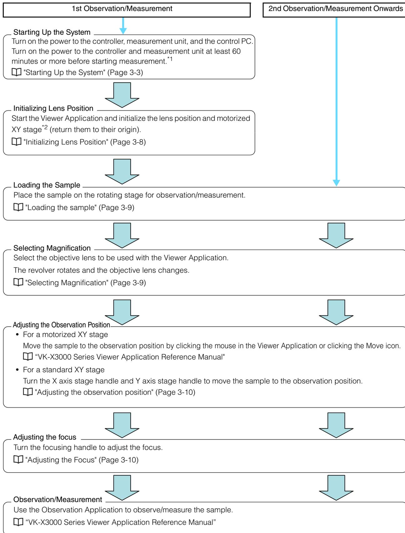
\*1 Wait one hour after turning on the power to the controller before taking measurements.
