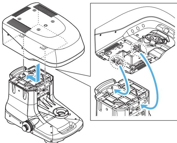
2 Secure the measurement unit to the base with the eight bolts.
