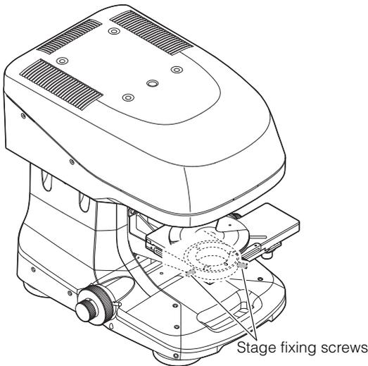
**NOTICE** The standard XY stage can accommodate samples up to 70 mm in height and 5.0 kg in weight.
