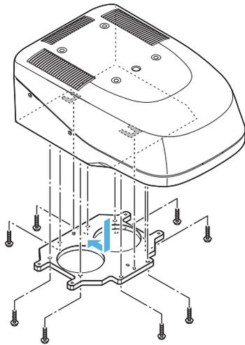
**3** Mount the bottom spacer and then the middle spacer to the base by aligning the positioning pin with the positioning hole and screw in six M6 20 mm bolts and six M6 35 mm bolts.
