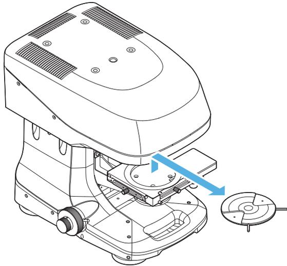
**2** Insert the protrusion on the base of the tilt stage into the recess in the center on the top of the XY stage.
