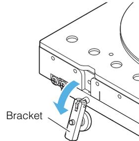
Removing the brackets allows the XY stage to move forward, backwards, left, and right.
