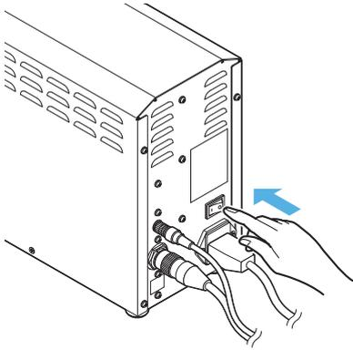
**Point** When the power LED on the front of the controller is lit in orange, the power is already on. You do not need to turn on the main power switch on the back of the controller.
