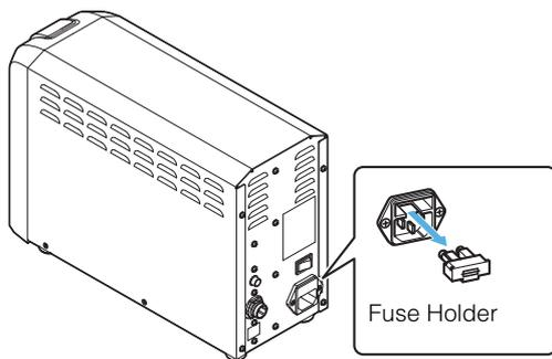
**4 Insert the new fuses into the fuse holder.**
