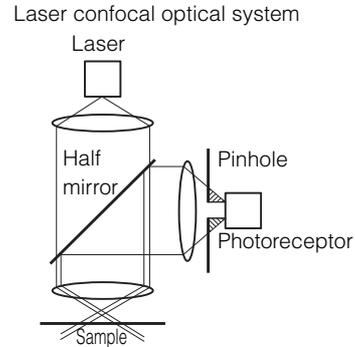
The height information (shape) of the object is captured by detecting the lens position in the Z axis when the reflected light intensity is at its peak.
