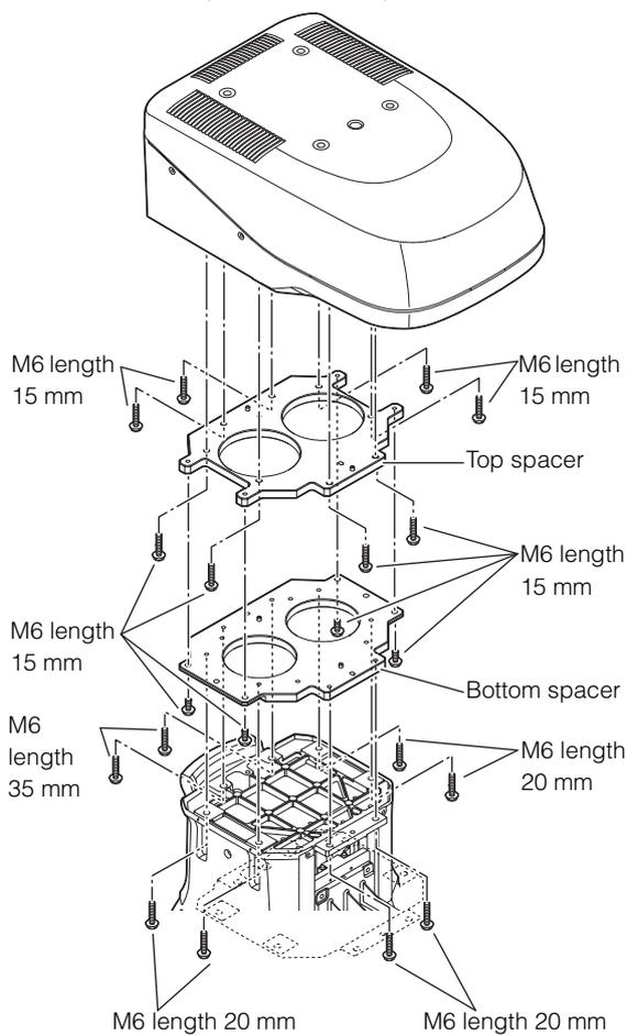
Adjusting the height by 100 mm: Top, middle, and bottom spacers
