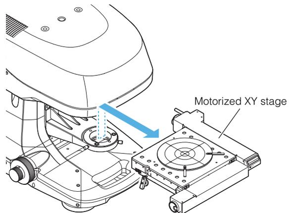
**4 Tighten the stage fixing screws.**
