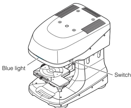
The power LED lights in blue. The controller power LED also lights in blue.
