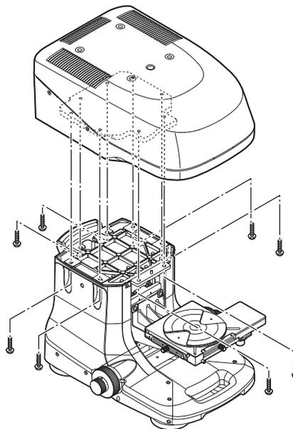
When mounting the measurement unit onto the base, be careful so that the measurement unit does not tilt over due to its weight.
