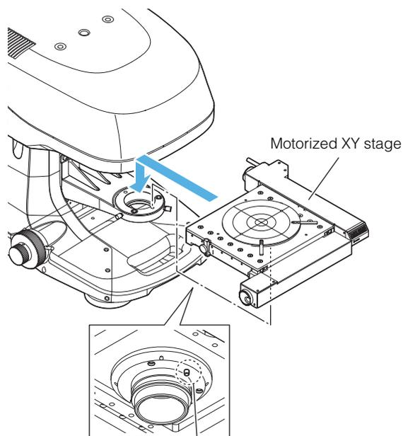
Align the pin with the stage hole position
