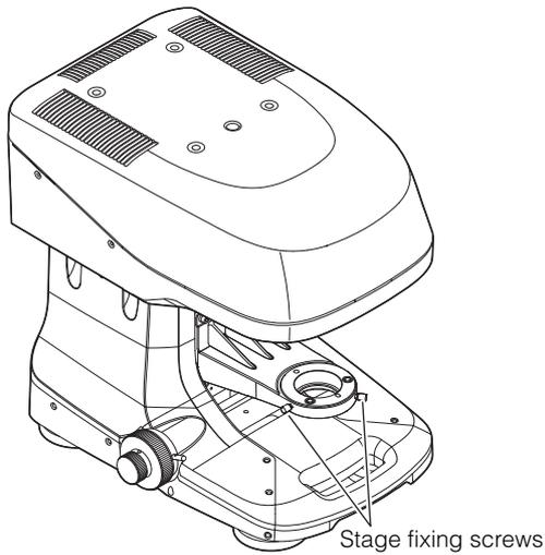
**3 Remove the measurement unit from the base.**
