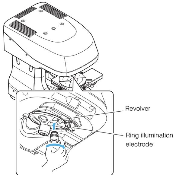
**NOTICE** Do not touch the ring illumination electrode when mounting the objective lens.
