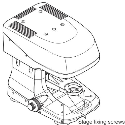
2 Remove the stopper ring from the bottom of the motorized XY stage and place the stage on the stage base.
