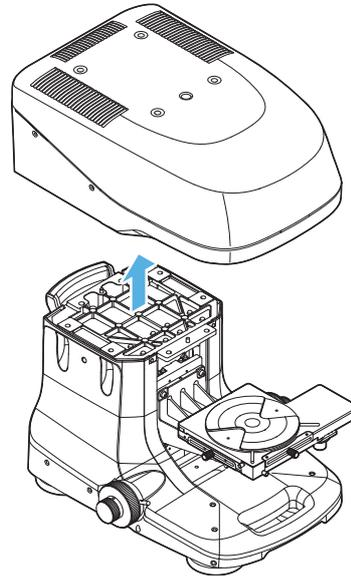
**Removing the Measurement Unit**
