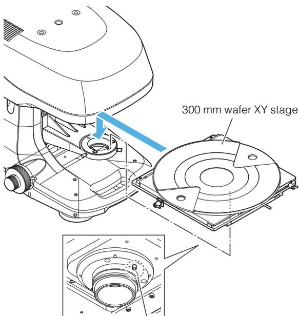
Align the pin with the stage hole position
