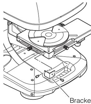
Removing the brackets allows the XY stage to move forward, backwards, left, and right.
