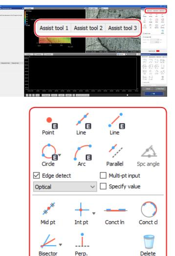
Assist tools such as points, lines, or circles can be used to assist in measurement.
