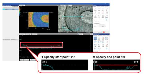
**3.** Draw another measurement tool [Red frame] on the profile graph, and measure the step.
