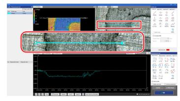
• Reference plane settings An object placed on the stage appears level to the naked eye, but to the microscope it is slightly tilted.
