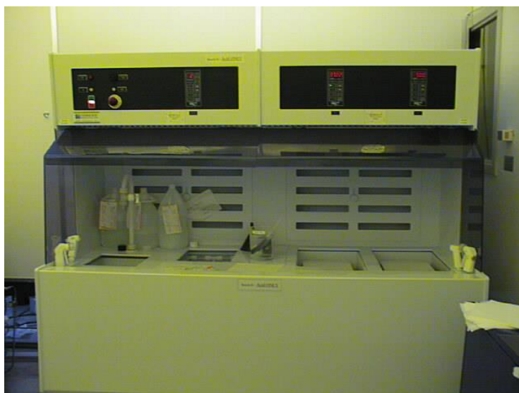
Acid hood, waste bottles in the back. Note – one sink/one user!
