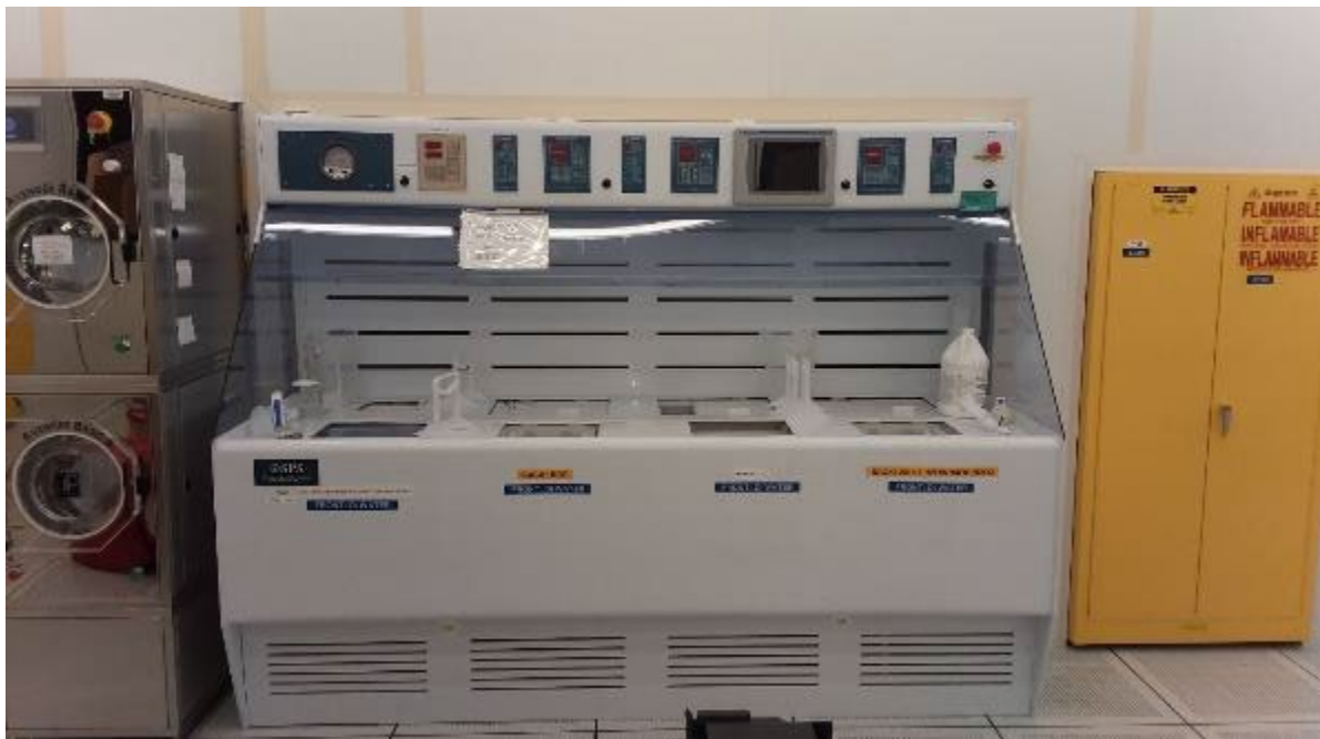
Acid hood, waste bottles and in use chemicals in the back. Note – one sink/one user and one sprayer/one user!
