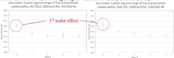
Once the 1<sup>st</sup> wafer is coated, the excess resist/solvent in the tray will cause the subsequent films to be thinner because of the higher solvent vapor concentration. For this reason, it is good to run a dummy wafer first, then run the device samples. For coating pieces, it may not be necessary to run a dummy wafer since the amounts of resist in the catch tray are minimal. Once again, it is up to the user to define the process conditions for their coating requirements.
