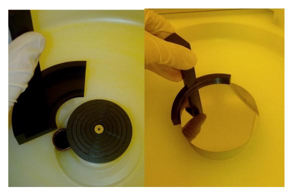
If it is a piece, the substrate will have to be manually centered before pressing the Vacuum "Hold" button
