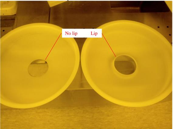
One with a lip on the inside opening and one without. The tray with the lip will catch and hold the resist directly under the spin chuck creating a very solvent rich atmosphere as more wafers are spin coated. This high solvent vapor environment may or may not help with your
