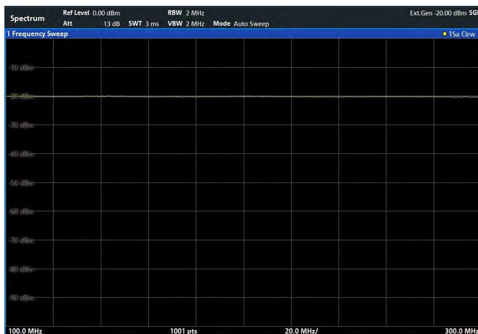
Figure 7-8: Measurement results from generator, analyzer and connecting cables
