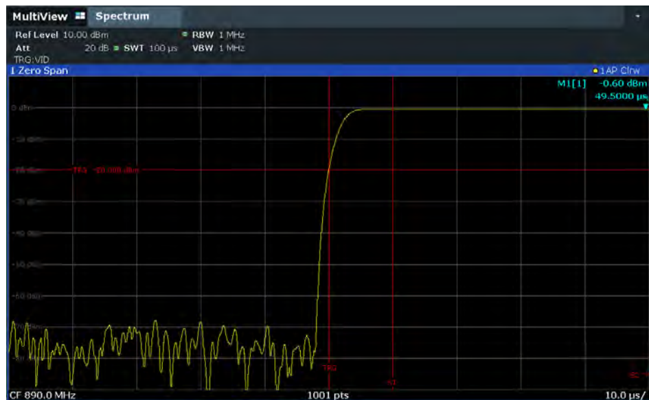
Figure 6-16: Rising edge of the GSM burst displayed with high time resolution
