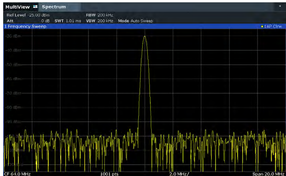
Figure 4-9: Calibration signal with optimized display settings
