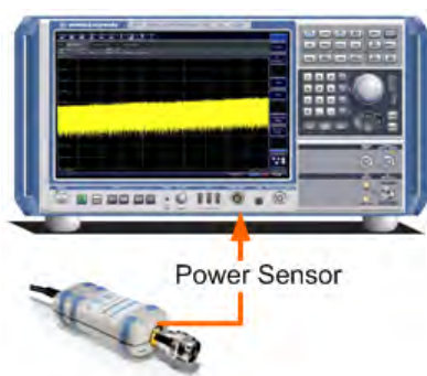
Figure 7-2: Connecting a power sensor using the POWER SENSOR interface
