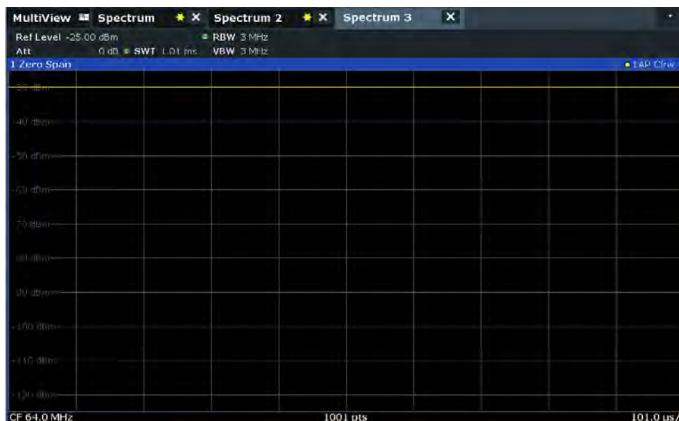
Figure 4-14: Time domain display of the calibration signal
