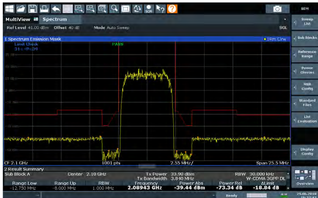
Figure 6-45: Detected peak display in SEM measurement
