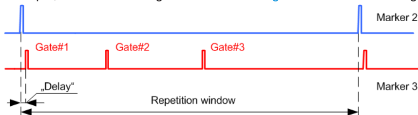
Figure 9-18: Marker signals used in multi-gated acquisition measurement
