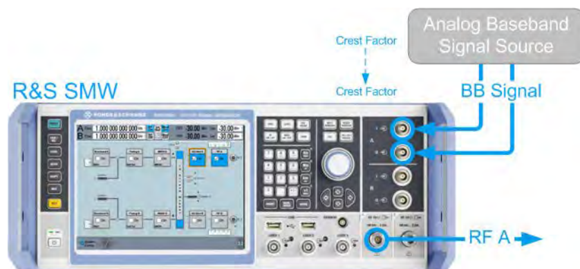
Figure 4-31: Example of test setup (simplified)
