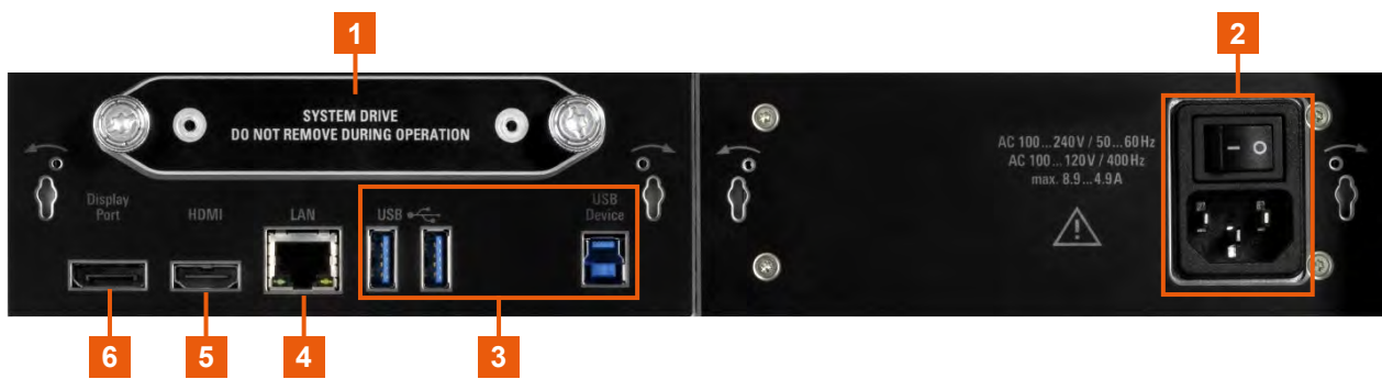
Figure 3-6: Processing board connectors and power supply
