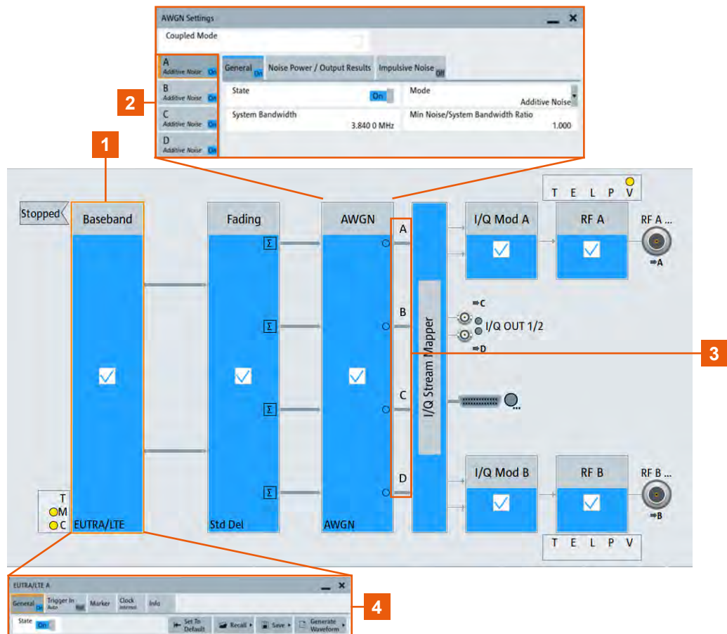
Figure C-2: Explanation of the naming convention for coupled sources
