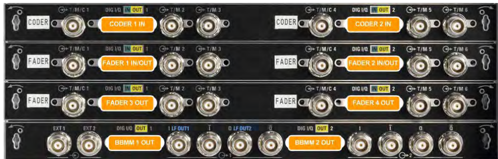
Figure 4-1: Standard baseband instrument rear panel: Digital input and output interfaces
