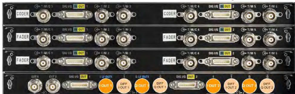
Figure 4-3: Standard baseband instrument rear panel: Analog output interfaces
