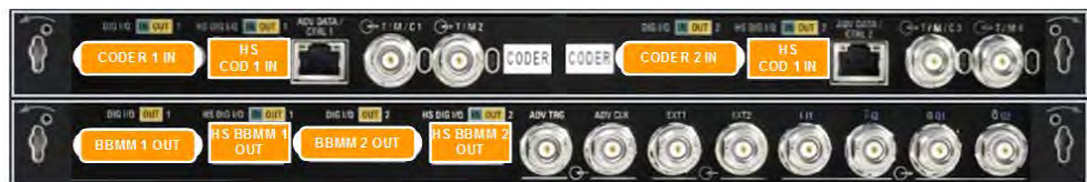
Figure 4-2: Wideband baseband instrument rear panel: Digital input and output interfaces
